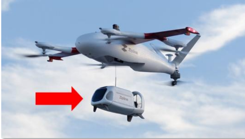
FIGURE 1: ZIPLINE P2 DRONE DELIVERY SYSTEM (ARROW POINTING TO "DROID")
